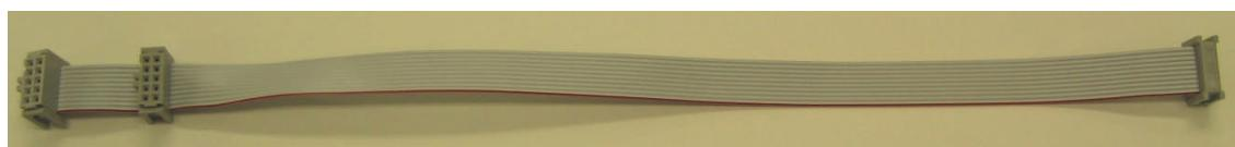
The Control bus and power are provided by a 10 wire ribbon cable that connects on the ALEX end to both 10 pin connectors, and on the other end, to the ten pin connector on the front of Mercury.
