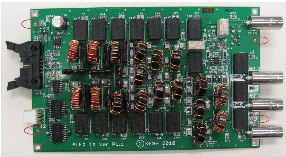
Optional holes for ground wires to housing ground shown inside red ovals.
