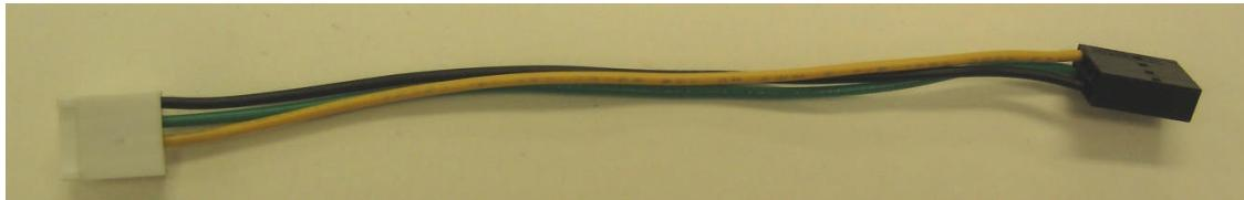
As an alternative to the RF Power cable supplied with the transmit board, the forward and reverse power voltage sense wires are also available on Pin 20 (forward) and Pin 7 (reverse) of the DB-25 connector.
