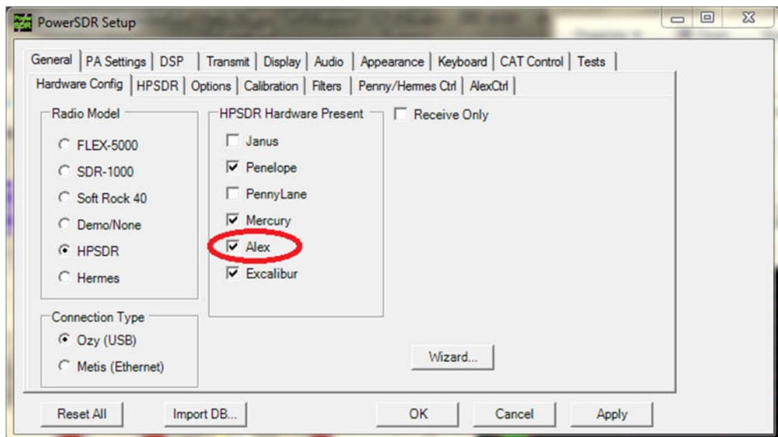
The Attenuator controls will now be integrated into the PowerSDR front panel controls for the Preamp. The menu will now allow you to select Attenuator settings of 0, 10, 20 and 30 dB in the Preamp window, in addition to turning the Mercury PreAmp On and Off.
