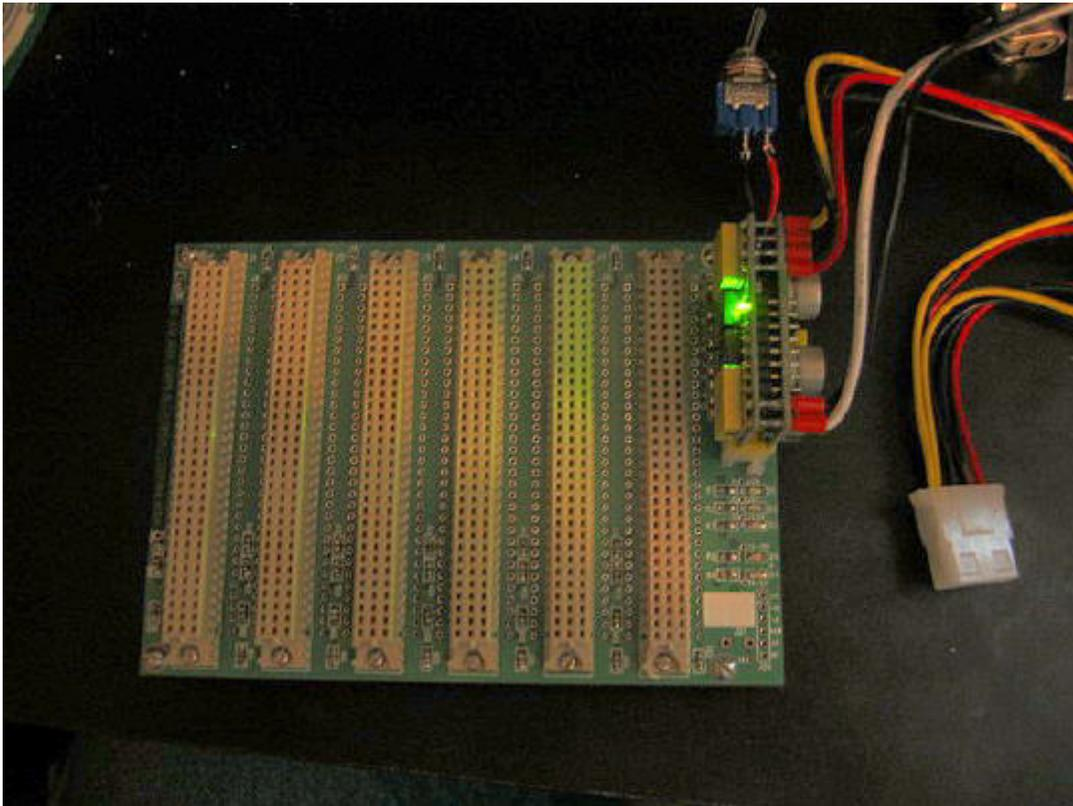
Assembled ATLAS with a PicoPSU ATX power supply plugged in
