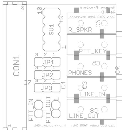
The 10-pin header (SV1) carries the 7 open-collector output signals on pins 1 through 7. The "open collector reference/flyback diodes" signal is on pin 8. Pins 9 and 10 (which are oriented nearest to the board edge) are ground.
