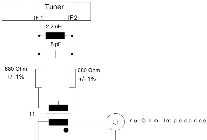
test circuit attenuation: 22.6 dB
