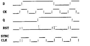
Next, the synchronized clock is applied to one input of EXCLUSIVE-OR gate 2, with the data applicate to the other input. The output is Manchester encoded data suitable for JAS-1.
