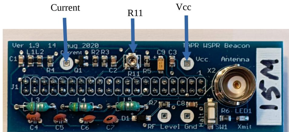
Figure 9: VW Transmitter Test Points and Current Adjustment
