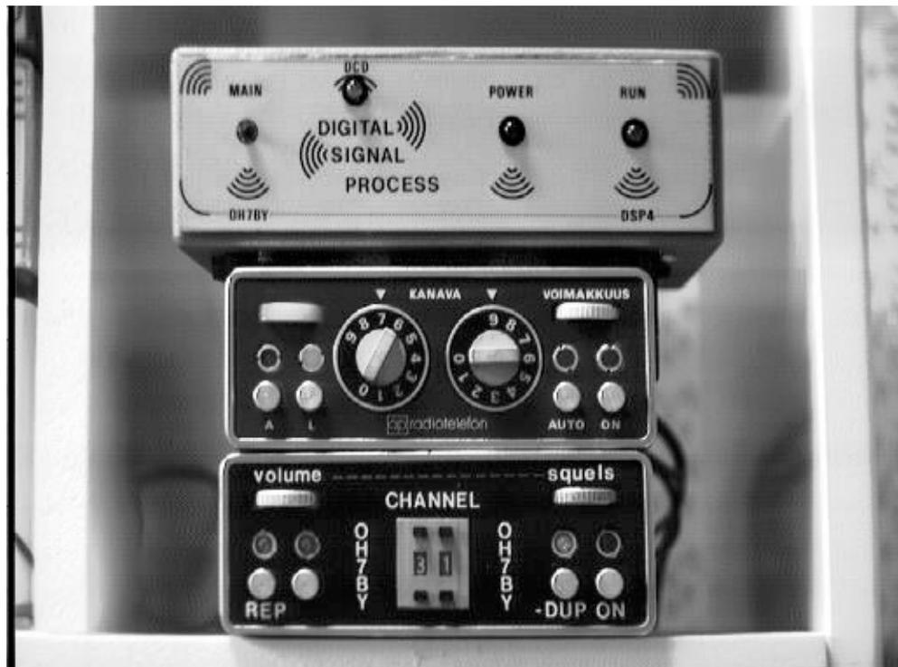
Figure 31: OH7BY's Satellite station with DSP CARD 4. At the top is DSP in a box, below is 2m transmitter and the lowest box is a 70 cm receiver. Both radios have previously been auto radiophones.
