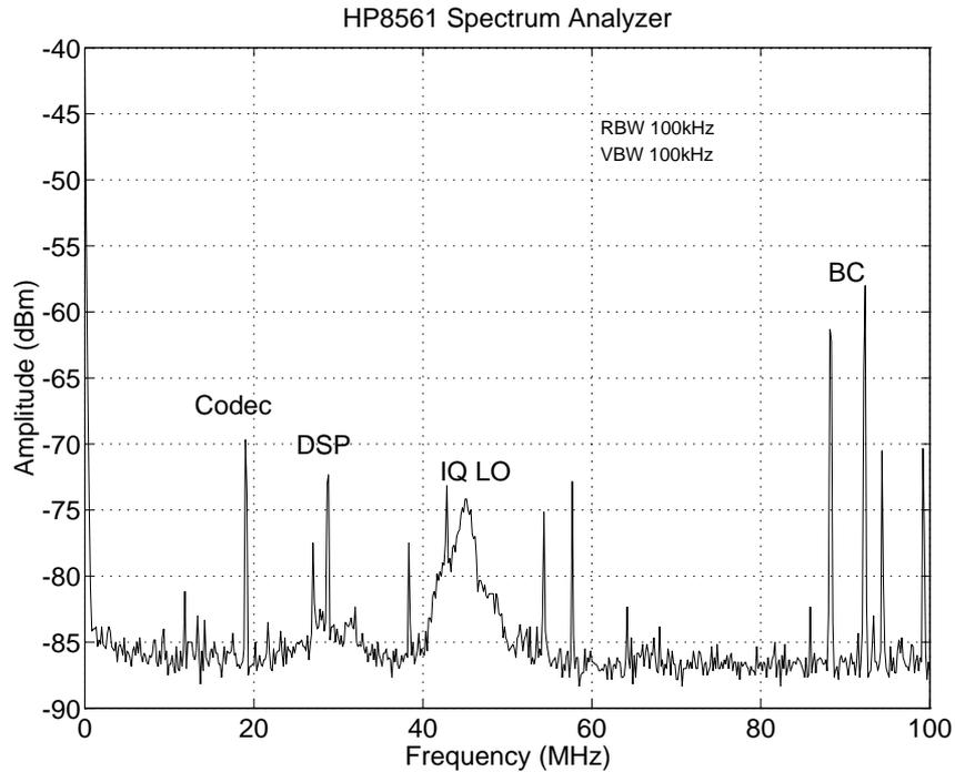
Figure 37: Noise spectra of DSP CARD 4 when in open environment.
