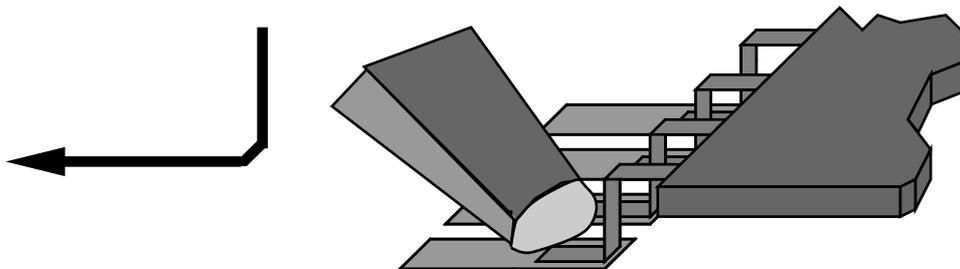
Figure 33: Soldering the DSP.
