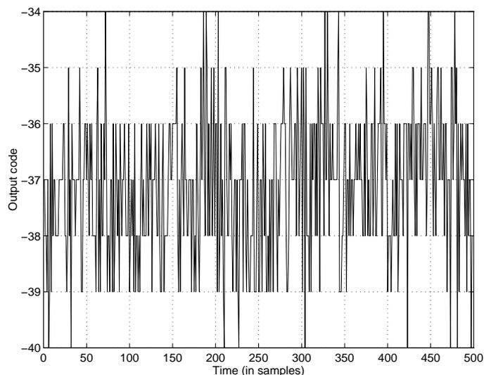
Figure 35: Output of the codec when the input is grounded and  $f_s = 48\text{kHz}$ .
