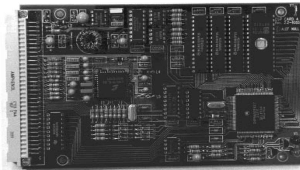
Figure 36: Figure of the first Rev 2.2 batch DSP CARD 4 PCB. We have CQFP version of DSP56001 on this first board, but PQFP is ok also (and it is cheaper).
