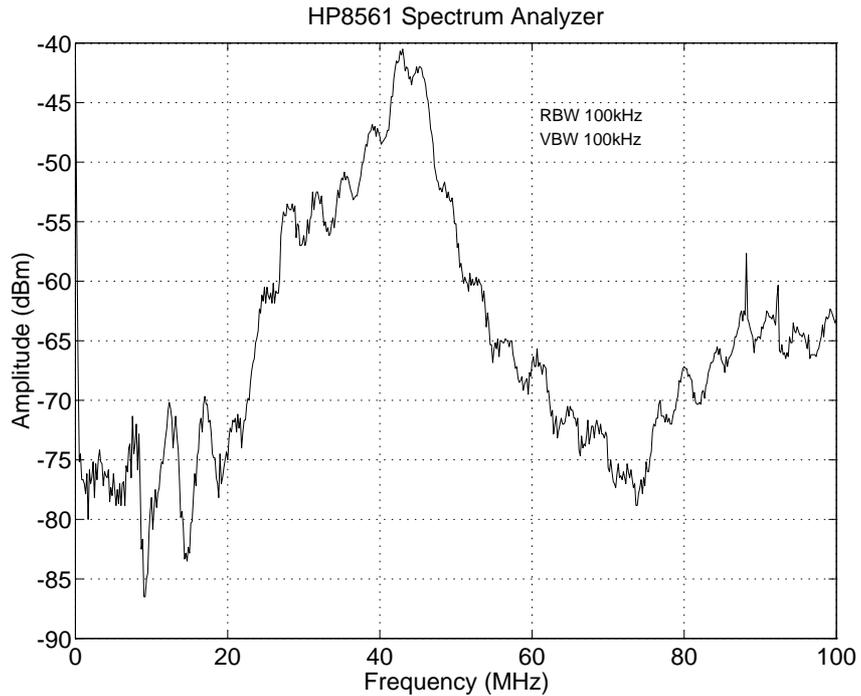
Figure 38: Noise spectra of DSP CARD 4 when in metallic box.
