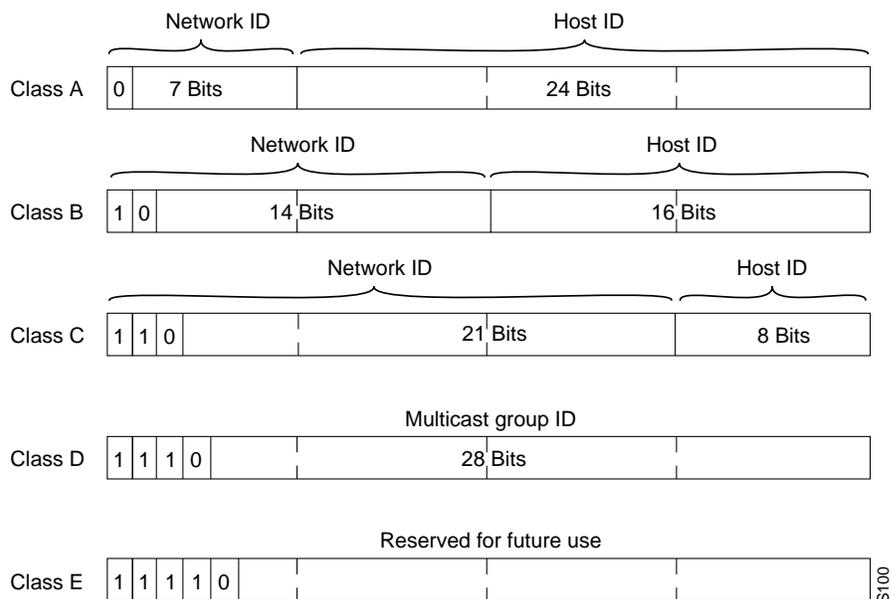
No matter which class of network you use, a host portion of all zeros indicates the network address. A host portion of all 1s (represented as 255) indicates the broadcast address. Therefore, the Class C address 192.168.180.0 is a network address, and the Class C address 192.168.180.255 is the broadcast address for that network.
