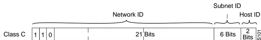
A subnet mask tells you how many bits to use in the subnet ID, and includes the number of bits in the network ID plus the number of bits in the subnet ID. For example, in a Class C network, if you use 4 host ID bits for the subnet, the subnet mask is 28. The dotted decimal format of this mask is 255.255.255.240.
