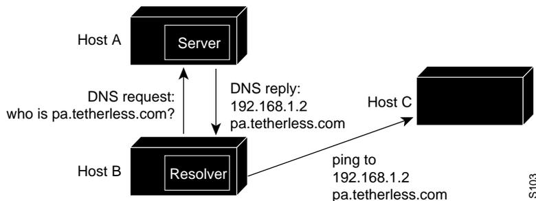
To take advantage of DNS, you must identify the domain name of the router you are configuring and the IP address of the name server you want to handle DNS requests. You can define multiple name servers to balance DNS requests.
