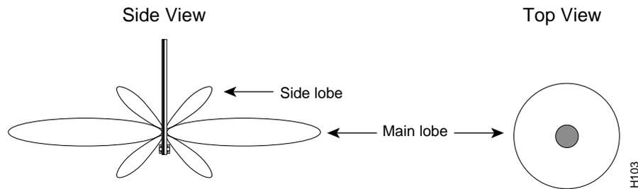
A directional antenna focuses RF energy in a specific direction. Ensure that you direct the antenna toward the opposite end of the link. Figure 2-2 shows a directional antenna. Use a directional antenna when making only a few links, the links are in similar directions, or you need more antenna gain to achieve an acceptable fade margin.
